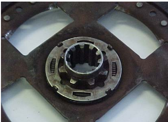
← Photo #3 Shows idle rattle cassette. Note springs at hub centre
