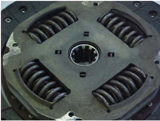
← Photo #1 Idle rattle suppression capable clutch plate
