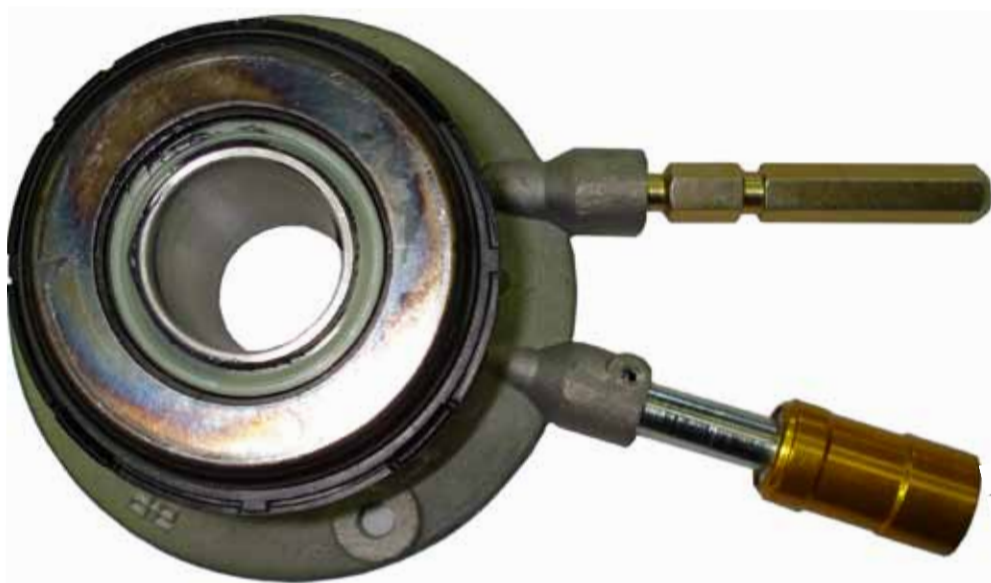
Design 1. Bayonet type delivery line.
